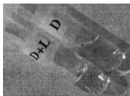
Figure 2. 12500-(PDLA 15 ) 2 13 wt% solution (D) and PEG12500-(PDLA 15 ) 2 + PEG12500-(PLLA 15 ) 2 13 wt% hydrogel (D+L) at room temperature.
